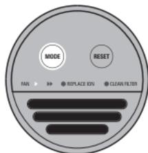
Push the Mode Button once. The unit will now run in **Low Output Mode**. (Denoted by One Arrow on Fan Speed Indicator)
